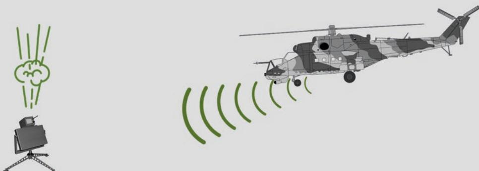
**PROTECTION AGAINST ANTI-HELICOPTER MINES: TRIGGERING PREMATURE ACTUATION**
