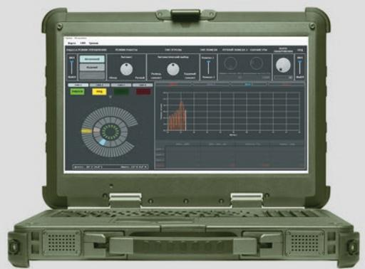
**RCS 'MIRAGE' ACTIVE JAMMER. CONTROL AND DISPLAY PANEL. OPERATOR WORKSTATION (OWS)**
