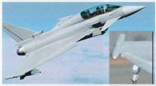
This artwork shows how the Talisman pods can be mounted on underwing hardpoints and can carry weaponry on their lower surface.
